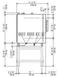
CWII Cold Water inlet 1 CWI2 Cold Water Inlet 2 Electrical inlet (power) Gas connection
